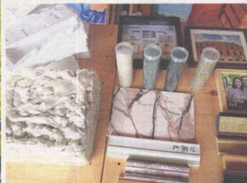
Bulky polystyrene from electronic goods packaging can be recycled into small plastic pallets and turned into picture frames, furniture and even solid walls.
