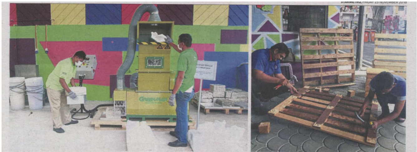
Bulky polystyrene from electronic goods packaging are being compressed to be made into useful items at the centre. — Photos: SAM THAM/The Star
